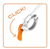
To unlock the double-leg kickstand, press the cockpit release lever until you feel it engage and hear a click.
