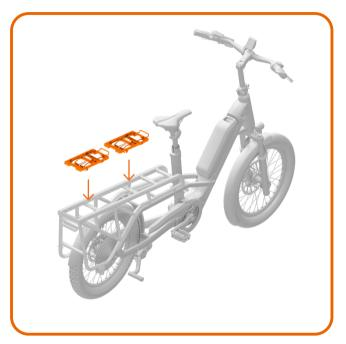
For assembly or disassembly, the 4 screws on each side must be fastened or loosened to do this; see page 29.
