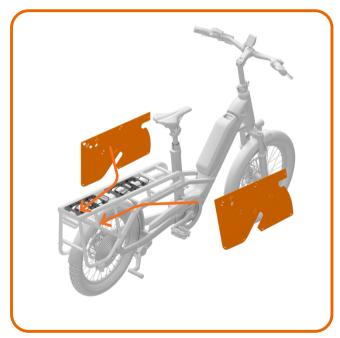
The wheel covers are pushed from front to rear between the rear wheel guard and the luggage carrier struts into the appropriate position. Use the holes for mounting the wheel covers (see image on page 31).
