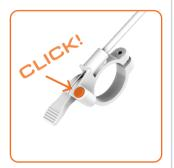
To lock the double-leg kickstand, press the button next to the release lever.
