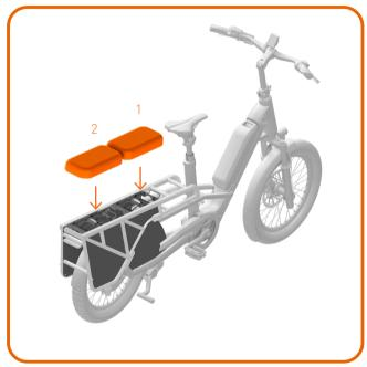
Observe the order in which the seat cushions are mounted on the MIK-HD system. Start with the front seat cushion. Disassembly is carried out in reverse order to the above.
