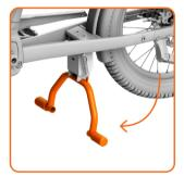
The double-leg kickstand is now unlocked and can be pressed onto the ground with your foot.
