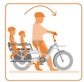
To fold up the double-leg kickstand, push your LOADY straight forward with some force. The double-leg kickstand folds back, up and away.
